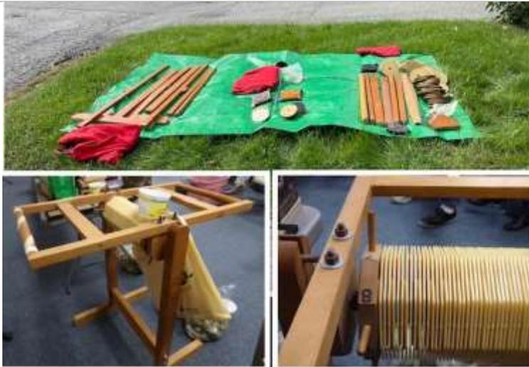
Weavermaster loom (mine is disassembled as shown in the top image; assembled, it looks similar to the photos shown below that. It operates by turning the cylinders in the middle which act in the same manner as shafts on a conventional loom, shifting various threads up or down to make a pattern). Comes in the 3 red cloth bags shown. Price: \$100
