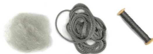
Conductive Materials for Spinning E-textile Yarns
