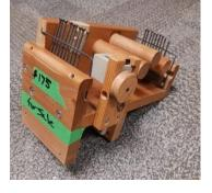
\*Tension Box\*–\$125 \$175 This is a tool that measures the length of the warp threads as you wind them onto the loom. It is usually used with a sectional back beam, allowing multiple threads to be wound from multiple cones/cores at the same time.
